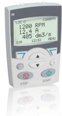
Assistant control panel
